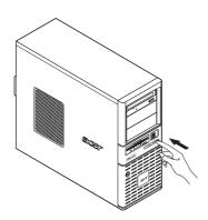
The system starts up and displays a welcome message on the monitor. After that, a series of power-on self-test (POST) messages appears. The POST messages indicate if the system is running well or not.
